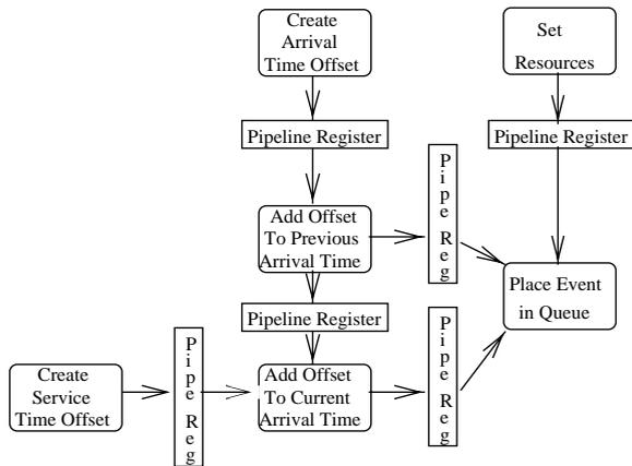
Figure 2: The Event Generator Flow Diagram
