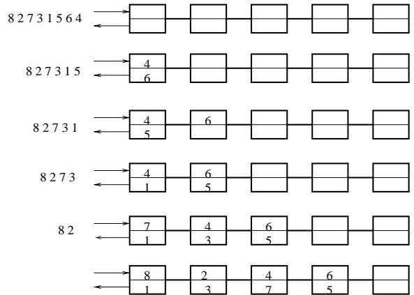
Figure 8: Linear Sort Array Input Example
