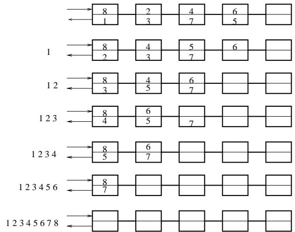
Figure 9: Linear Sort Array Output Example
