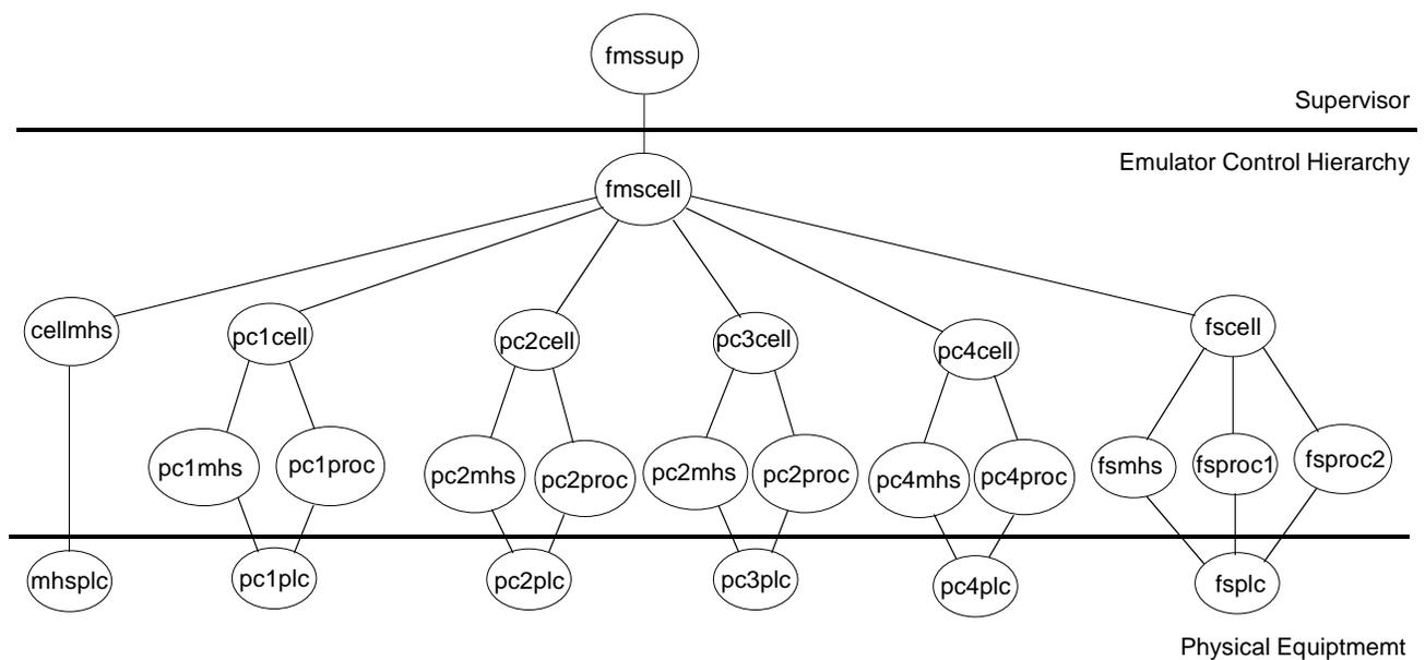
Figure 5. The ROOCH Decomposition of the Model Used to Control the Emulator
