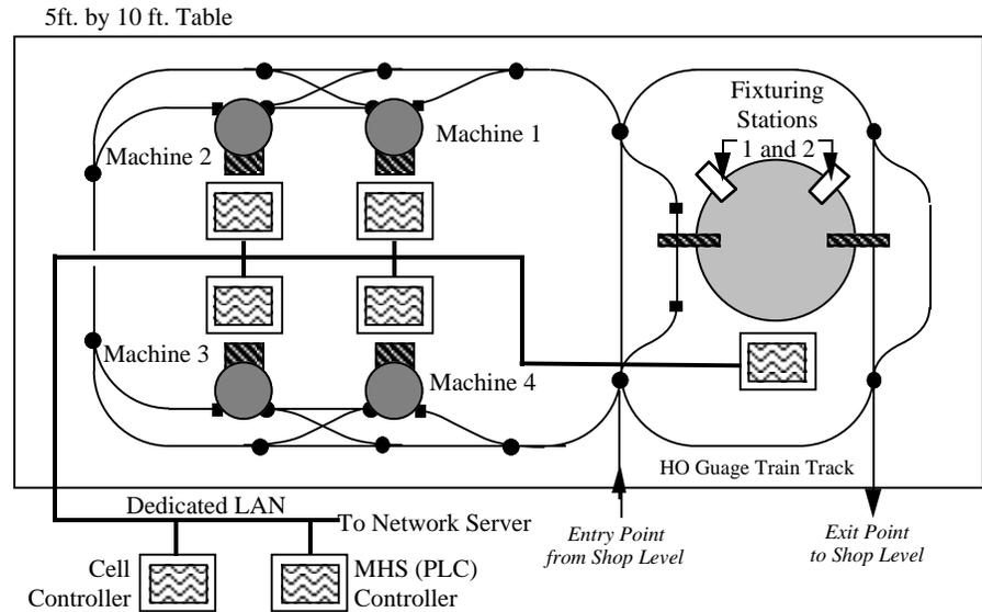
Figure 2. Schematic for the Layout of the Physical Emulator
