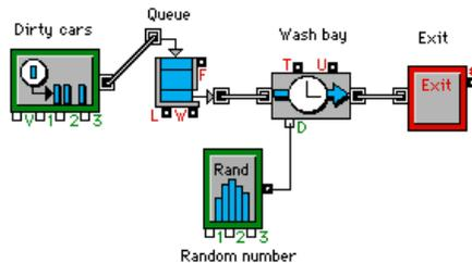
Figure 3: A Model with Random Process Times
