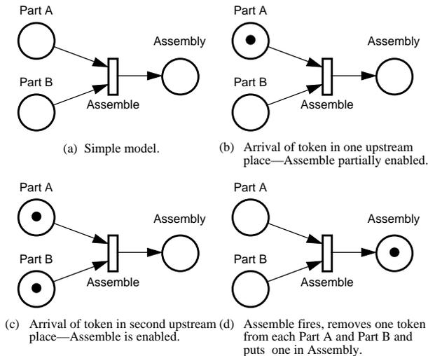
Figure 2: Transition Firing
