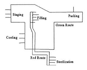
Figure 1- AGV Path Layout
