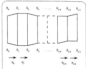
Fig. 1: Discrete two-dimensional height-field representation of the water surface h, the ground bottom b, and the horizontal water velocity u
