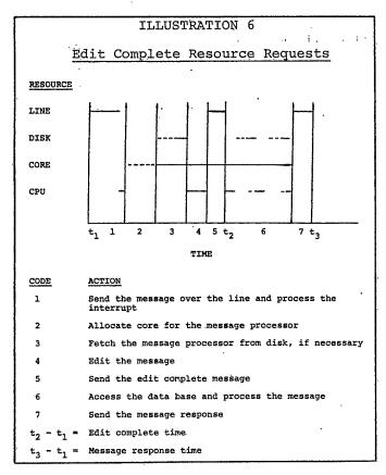
among the experiments. The dashed lines represent queueing delays for the resources. The variability in these delays (codes 2 and 3) plus the frequency of program fetches caused the variability in edit complete times.
