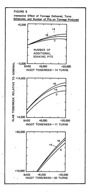
factor. At 17 turns, increases in the rolling rate at the higher delivery levels produce additional tonnage. At low delivery levels, increasing the rolling rate above 9 tons per minute has little or no effect because all or almost all of the delivered tonnage is being processed, even at the slower rate. The effect of rolling rate is less pronounced with the 20-turn operation because the greater availability of the rolling facility is the overriding factor.
