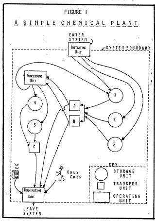
This plant has five storage units designed as STUI through STU5. These are aggregated into storage unit groups and areas shown in Tables 1 and 2. Note that since the order in which we consider the storage units is important, group STU-GRP3 consists of storage units STU4, STU5, and STU1, not STU1, STU4, and STU5. Materials are stored in the storage unit groups indicated in Table 3.
