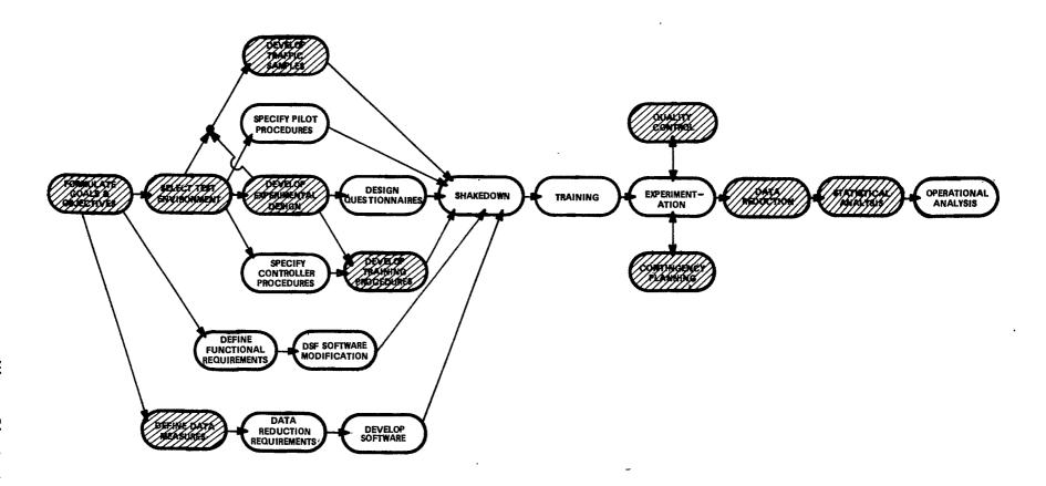
FIGURE 1 SCHEMATIC DIAGRAM OF DSF PROJECT ACTIVITIES
