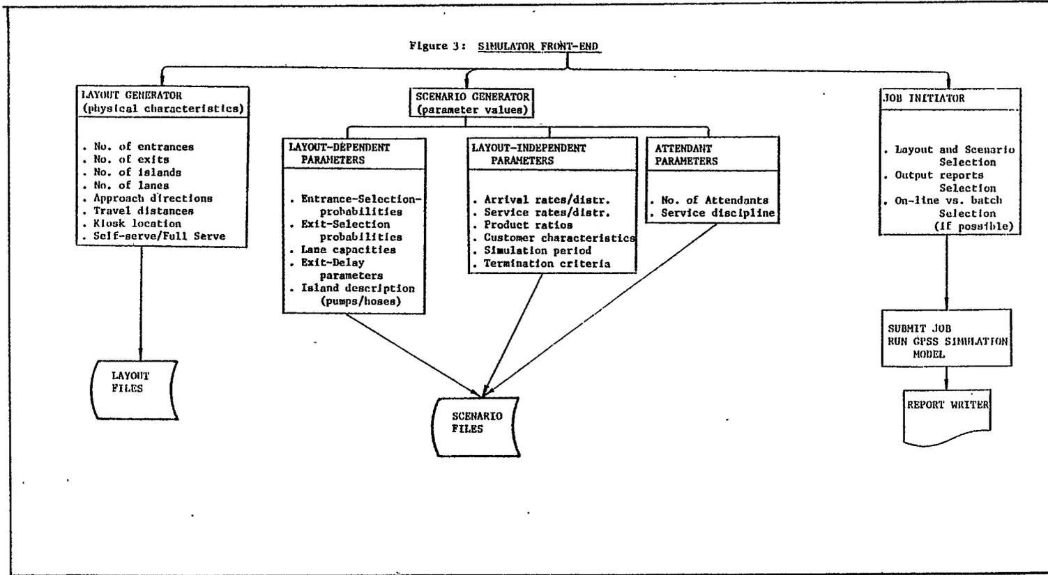
control of a user-specified function. At the beginning of each hour, the model will refer to the function and calculate inter-arrival times corresponding to the requested number of arrivals. If the station is already operating at capacity (also user-defined) excess customers are designated as 'drive-aways'.
