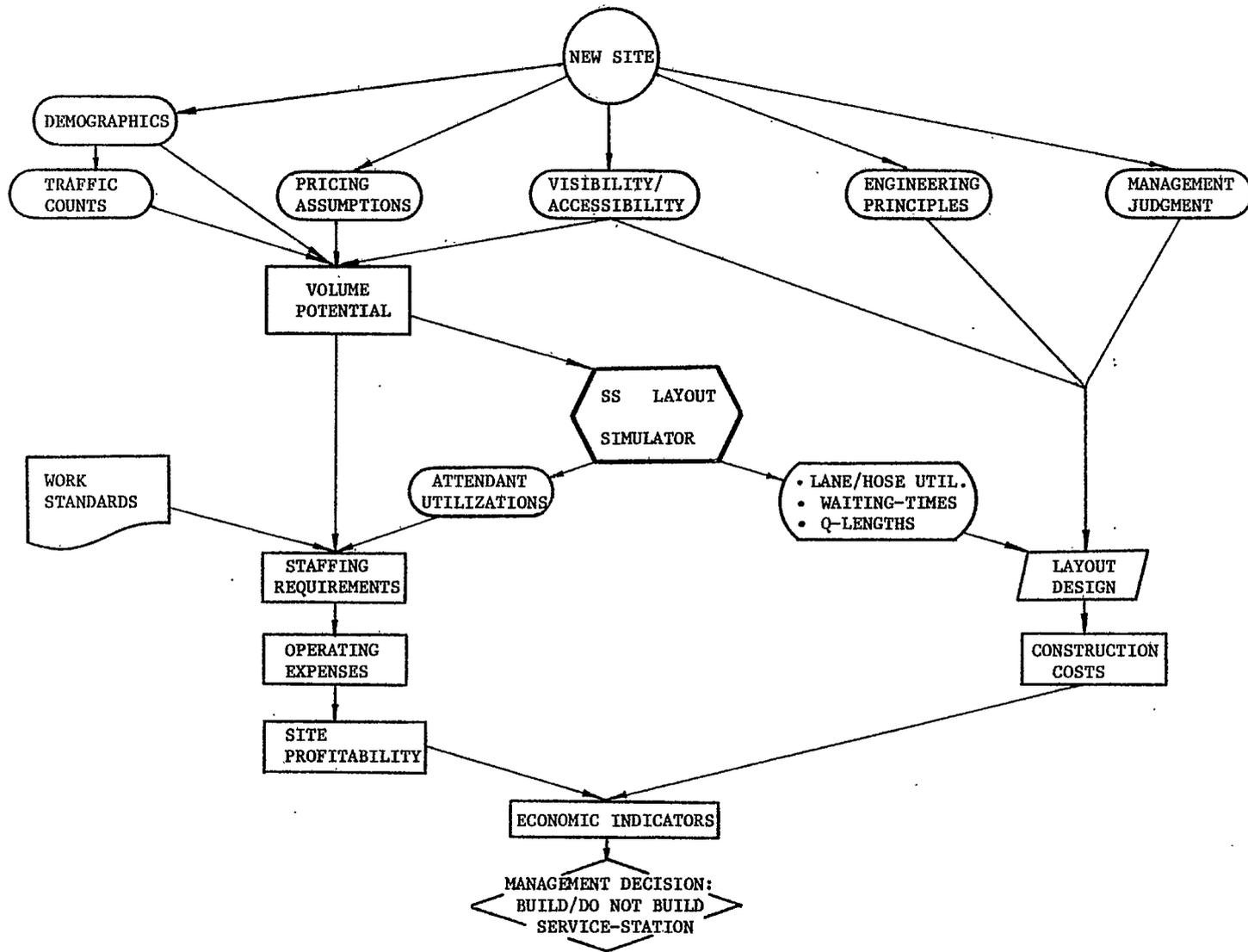
FIGURE 1: ROLE OF THE SS LAYOUT SIMULATOR IN THE NEW-SITE EVALUATION PROCESS
