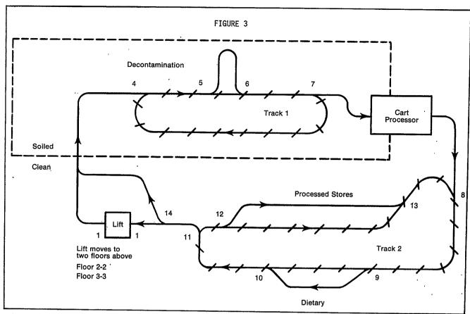
the exit queue will hold six carts. On the user levels where no monorail system exists, the entry queue is restricted to one cart. The exit queue however, is specified to hold a maximum of two carts. When this queue becomes full, the lift will not eject another cart at this location but will stop at this location and go into a holding mode.
