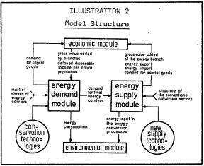
gives an overall view of the links between these modules, which form an interaction structure of closed-loop type.
