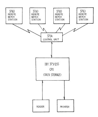
Figure 2. Equipment Considered Within the Model.
