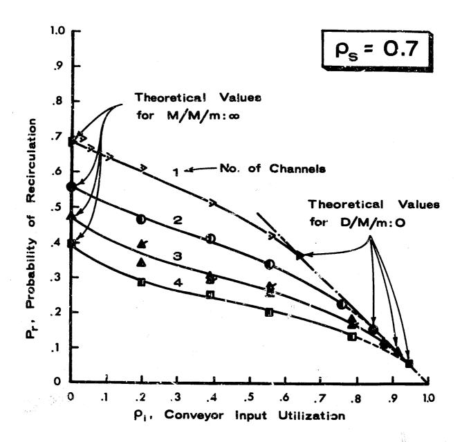
Figure 4. Effects of Conveyor Input Utilization and Number of Chennels on the Probability of Recirculation.
