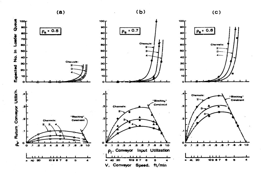
Figure 3. Effects of Conveyor Input Utilization, Conveyor Speed, and System Traffic Intensities on Basic Operational Characteristics.
