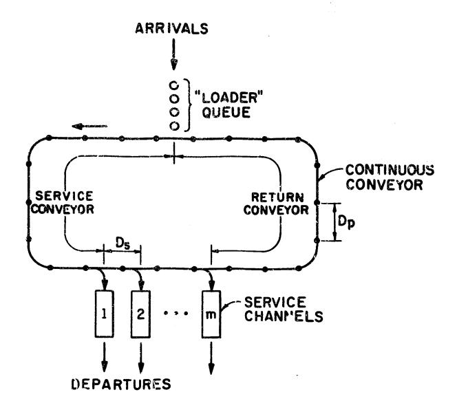
Figure 1 - Conveyor-Supplied Multiserver System.
