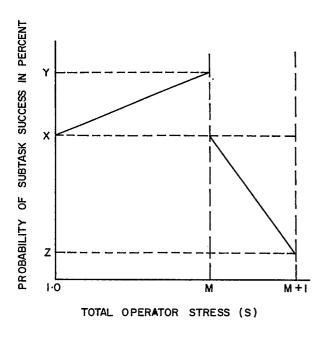
FIG. 4: Subtask Success vs Operator Stress
