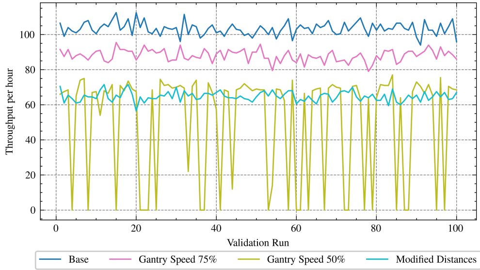
Figure 3: Results of validation runs for the base model II (3 H-style gantries; 5 process steps) with gantry variations .
