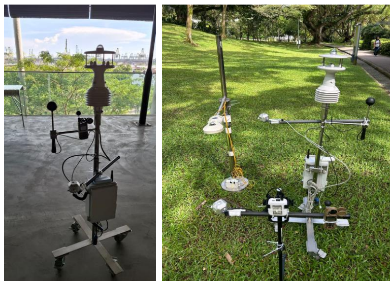
Figure 7: The mobile weather station (left) and measurement comparison with static sensors (right).
