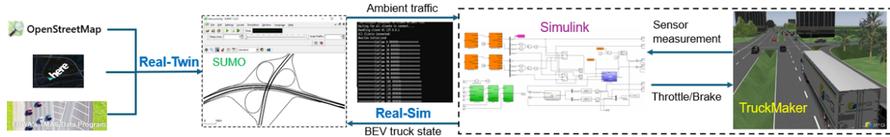
Figure 1: Co-simulation framework between SUMO and IPG TruckMaker TM
