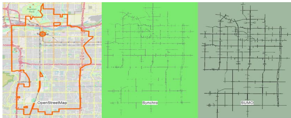
Figure 6: Network for Tempe, AZ, shown in OpenStreetMap, synchro network, and SUMO network.
