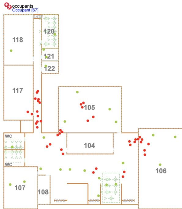
Figure 1: Floorplan of the building simulated and an example of simulation run (green dots represent agents who secure the physical distance and red dots represent occupants who violate the physical distance).
