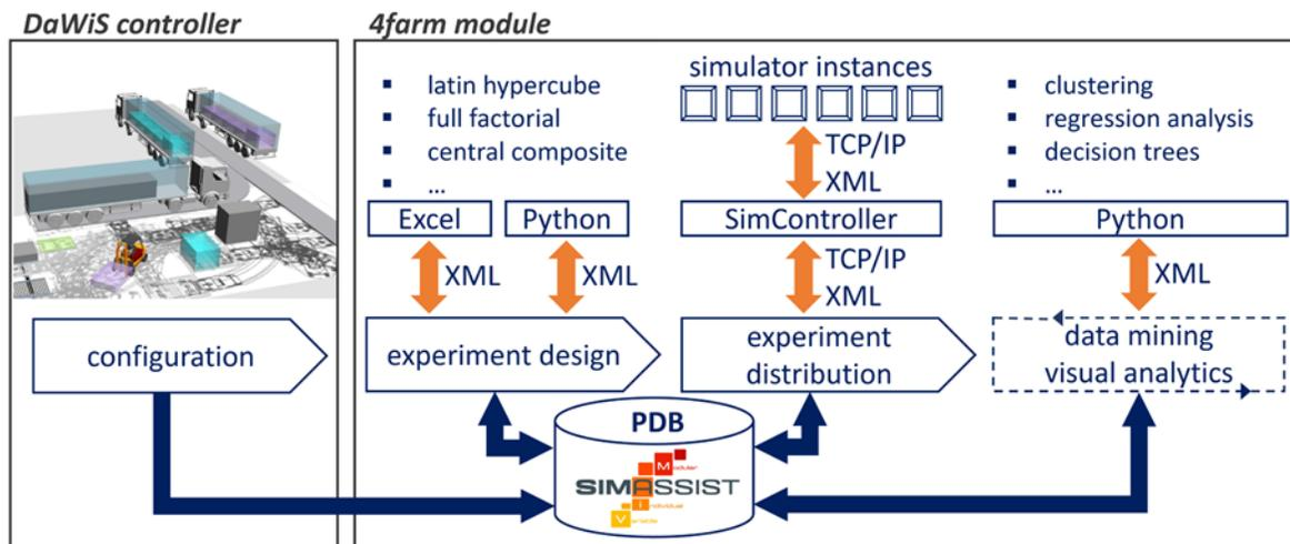
Figure 1: Conceptualization of the integrated solution for data farming and knowledge discovery.
