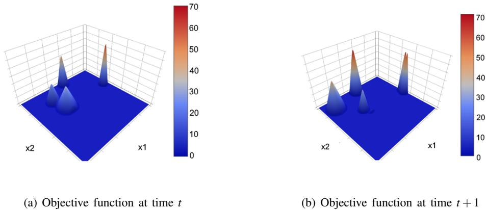
Figure 3: Behavior of a dynamic optimization problem. Over time the different optima can move, grow or shrink.
