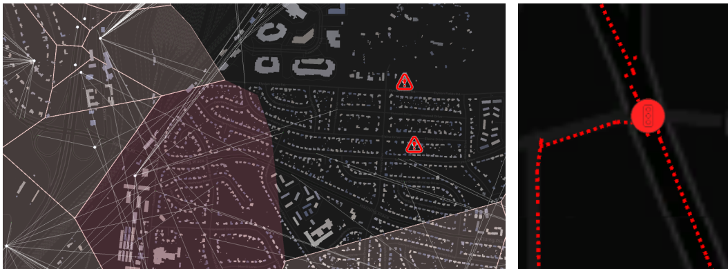
Figure 1: Example images of effects of a power failure cascade. The left figure shows the effect of two disabled cell phone towers (red triangle exclamation points, dark regions represent those cell towers service area) overwhelming an adjacent cell phone tower (medium shaded area). The right figure shows cars (red squares) backed up at an intersection with a disabled traffic light (red circular disk).
