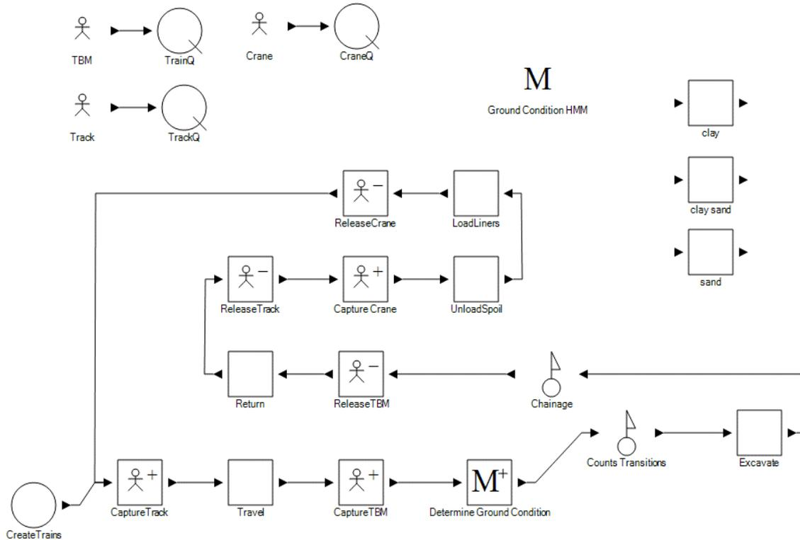
Figure 3: Case study tunneling model schematic.
