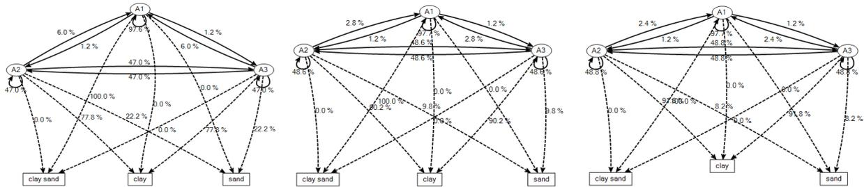
Figure 5: HMM chain for runs 1, 5, and 6 (from left to right, respectively).
