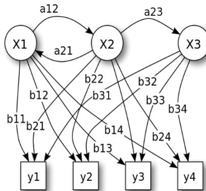
Figure 1: Graphical example of a HMM, where (x) represents a hidden state, (y) represents an observable state, (a) represents a transition probability from a hidden state to another, and (b) represents the emission probability from a hidden state to an observable state.
