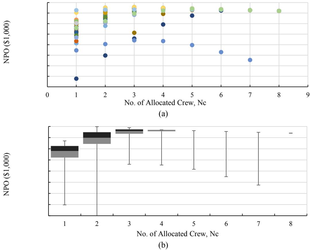
Figure 3: Change for *NPO* with different crew number for 30 independent MC run, (a) the cluster of *NPO* values for corresponding *Nc* value, (b) the box plot for each *NPO* data group.
