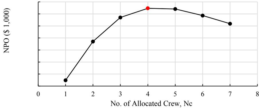
Figure 4: Lower bound of the 95% confidence interval of Net Production Output, (*NPO*) values for different crew number (*Nc*).
