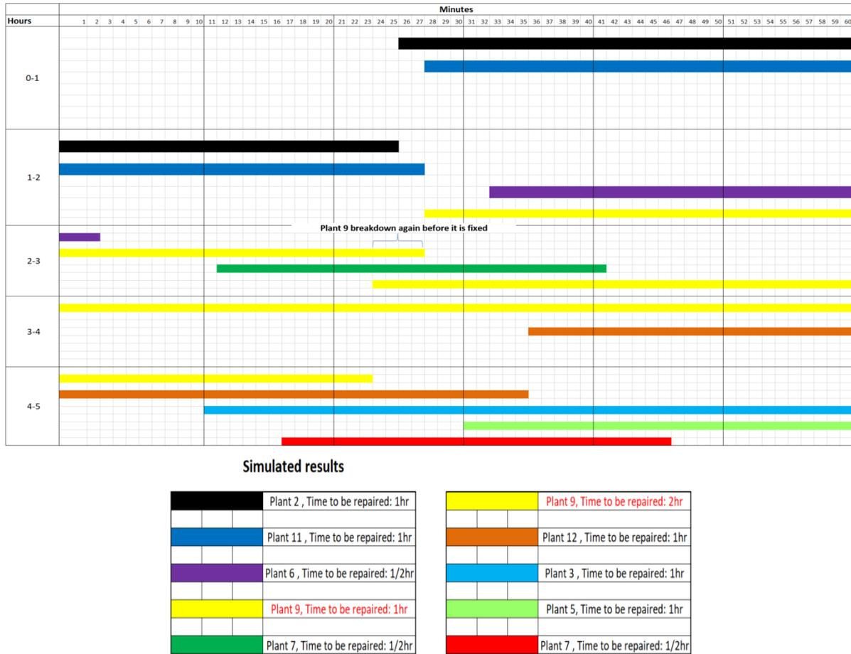
Figure 1: Plant breakdown simulation bar chart from one run over five hours.
