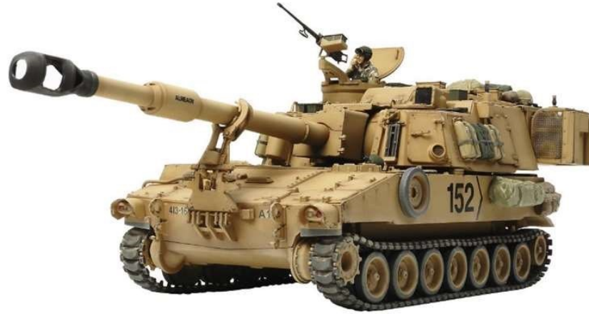
Figure 1: M109A6 Paladin is a self-propelled 155 mm howitzer and serves as the main firing system for mechanized field artillery units.
