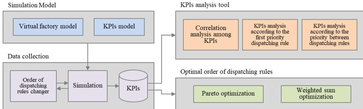
Figure 3: KPI analysis framework with multiple dispatching rules.
