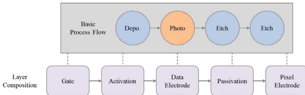
Figure 2: TFT shop process in the LCD fab line.
