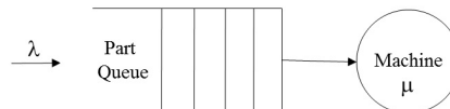
Figure 1: Single-stage production system with part arrival rate \lambda and part processing rate \mu .
