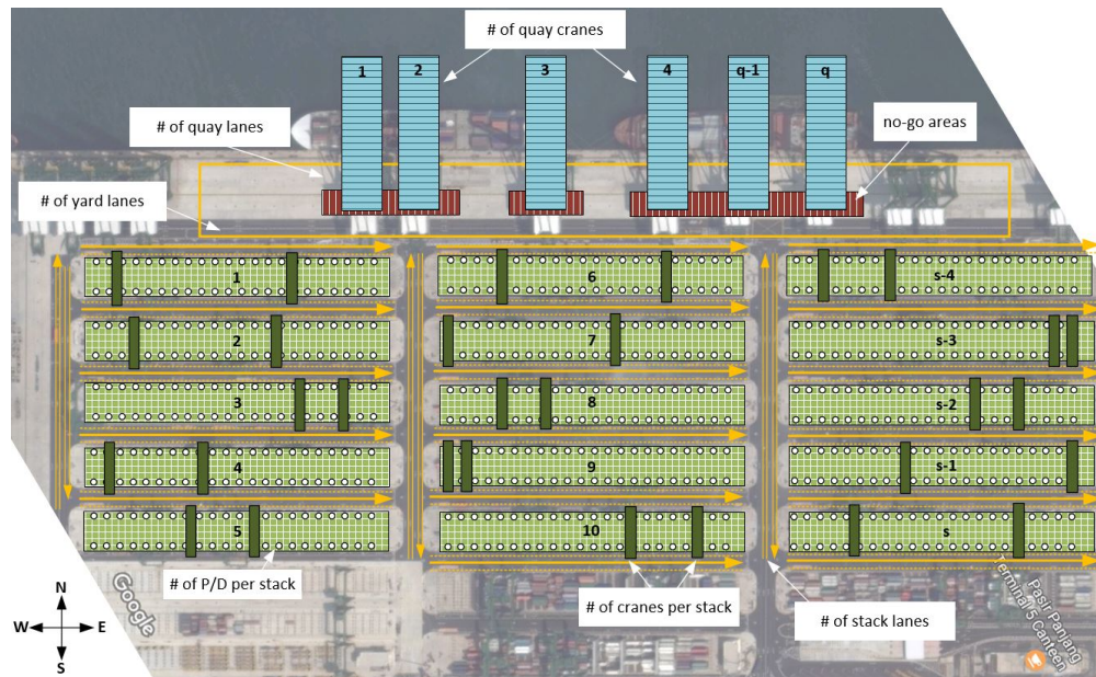
Figure 2: Top-down view of a container terminal in parallel layout.
