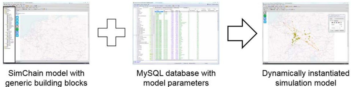
Figure 2: Working principle of the simulation tool SimChain (Rabe et al. 2017a).
