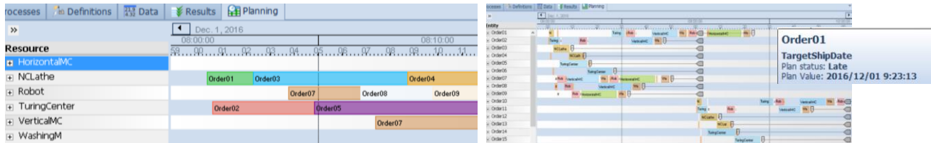
Figure 6: The Gantt chart of the Resource Plan (left) and the Entity Work Flow (right).
