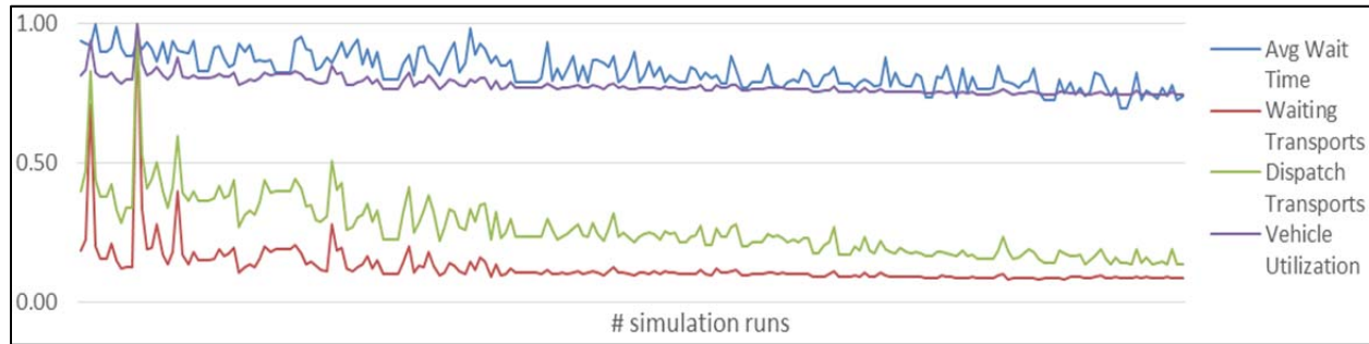
Figure 5: Development of performance parameters during optimization with GA to find suitable parameter sets (with normalized values).
