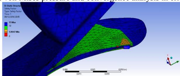
Figure 21: Safety factor value in critical case 3.
