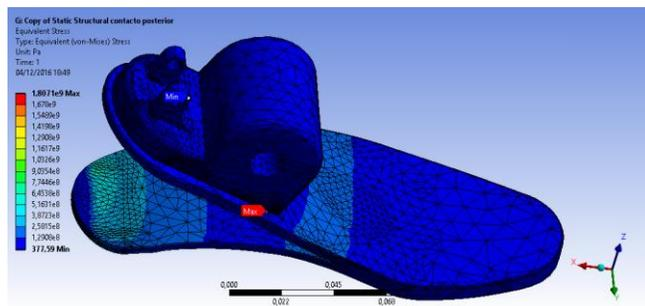
Figure 13: Maximum and minimum pressure value of von Mises.
