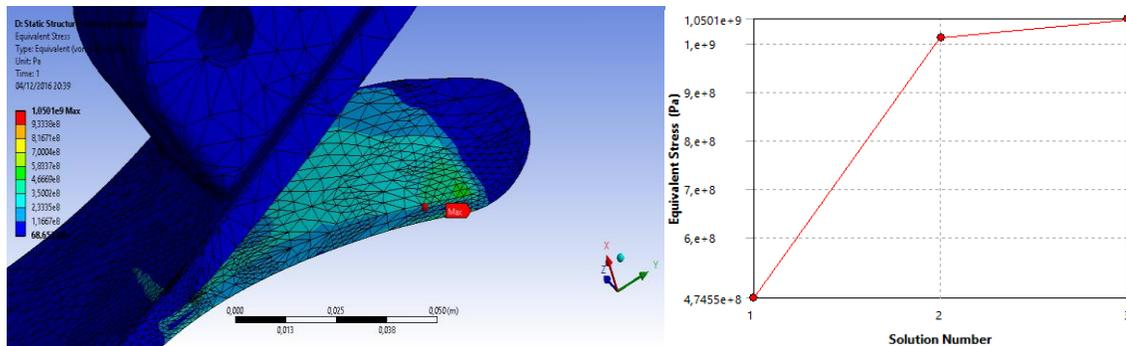
Figure 20: von Mises pressure and convergence analysis in critical case 3.
