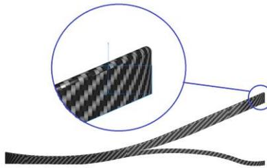
Figure 15: Increased thickness of 5 mm in the plantar base.
