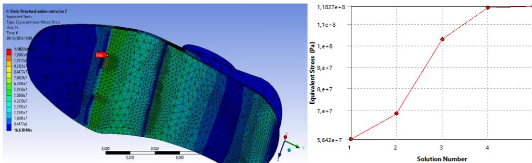
Figure 16: von Mises pressure and convergence analysis in critical case 1.
