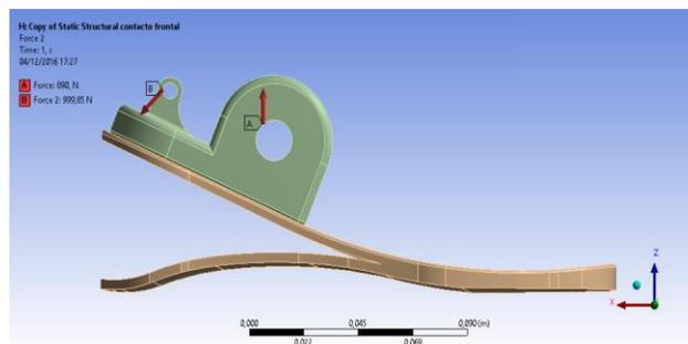
Figure 8: Loads acting on the prosthesis.
