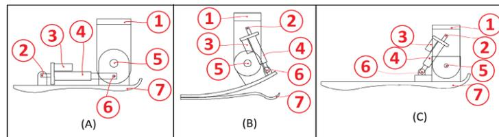
Figure 2: Sketches of prosthesis of lower limb, (1) Support for socket, (2) Upper joint of linear actuator, (3) Electric motor, (4) Recirculating ball screw, (5) Ankle joint, (6) Linear actuator lower joint, (7) Plantar base.
