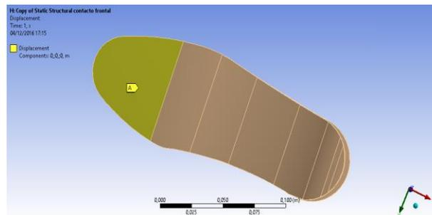
Figure 6: Displacement constraints in critical case 2.
