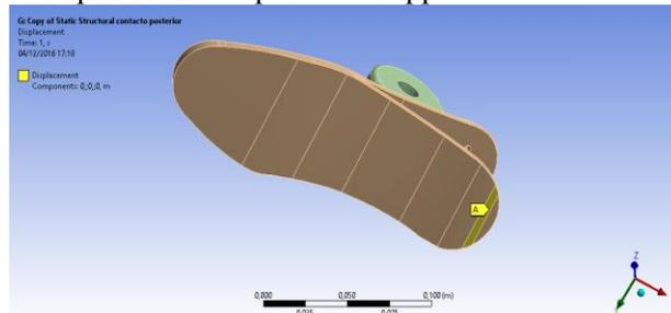
Figure 7: Displacement constraints in critical case 3.
