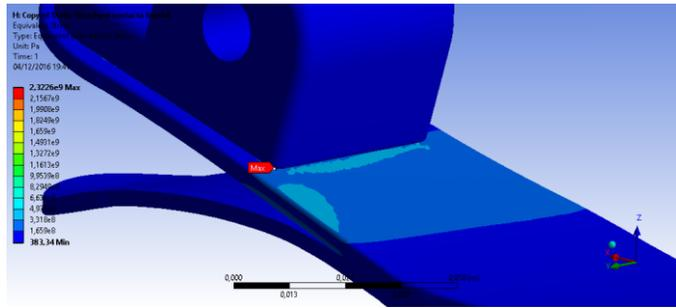
Figure 11: Maximum and minimum pressure values of von Mises.
