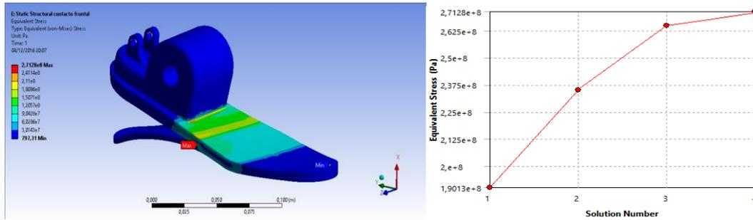
Figure 18: von Mises pressure and convergence analysis in critical case 2.
