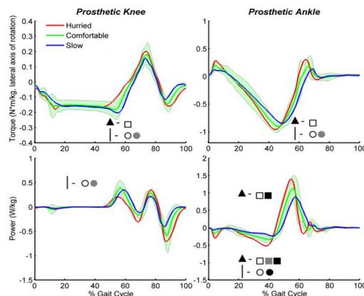
Figure 1: Torques and powers of knee and ankle during the walk on a slope. The shaded portion represents the standard deviation of the comfortable walking condition. The torque of the knee in terminal position and a maximum torque of plantar flexion of the ankle are compared as well as the power of the knee and ankle.
