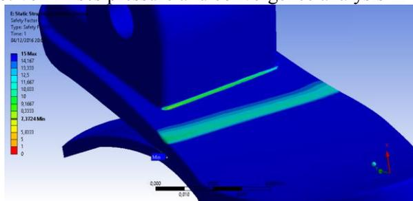
Figure 19: Safety factor value in critical case 2
