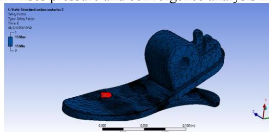
Figure 17: Safety factor value in critical case 1.
