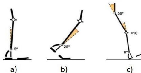
Figure 4: Critical conditions of gait cycle, a) total support of the plantar base, b) frontal support of the plantar base, c) posterior support of the plantar base.
