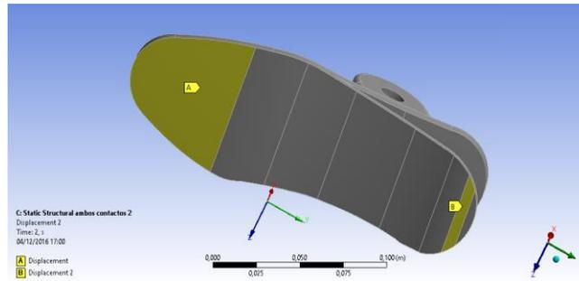
Figure 5: Displacement constraints in critical case 1.
