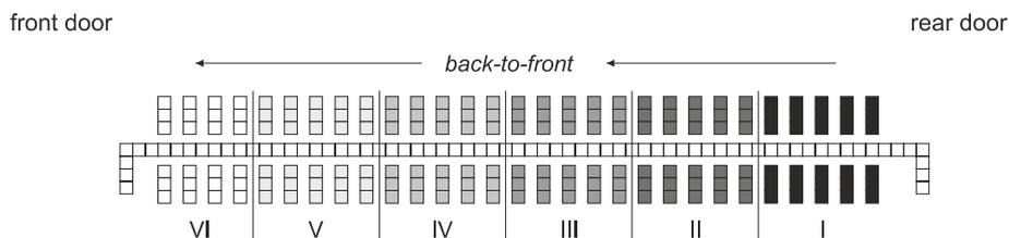
Figure 2: An example for *block* boarding strategy modelled in the simulation environment (darker seats are boarded first, this case results in a *back-to-front* regime).
