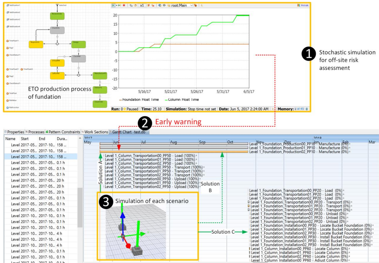
Figure 9: An on- and off-site logistics simulation example of bucket foundation and column.
