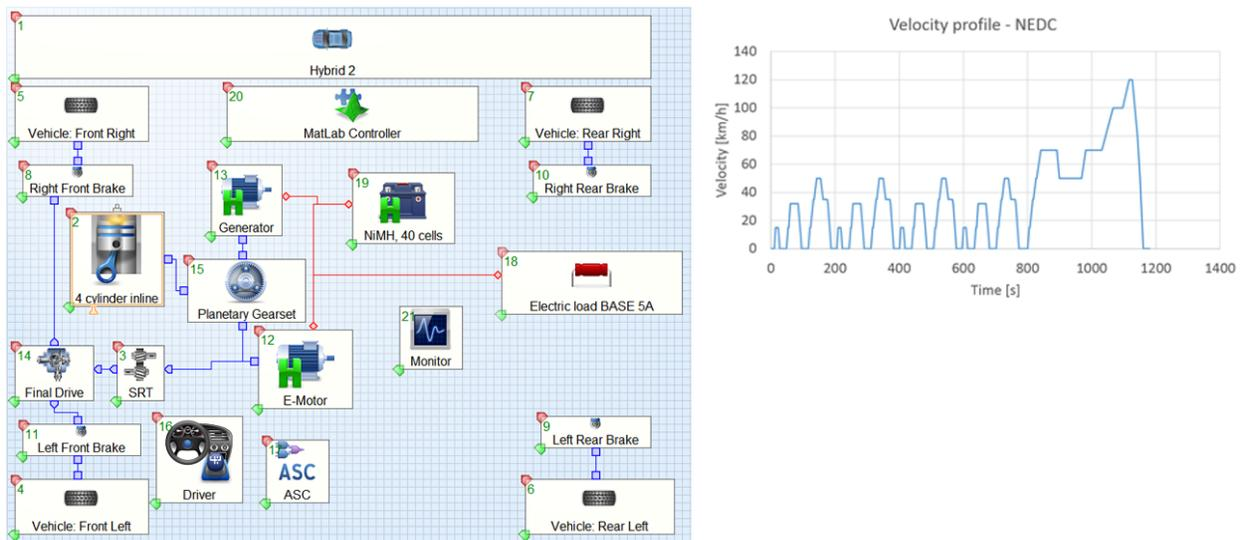
Figure 2: **Left:** The studied AVL Cruise simulation model. **Right:** A line chart showing six properties during a Cycle run test on the standard NEDC (New European Driving Cycle) velocity profile (1,180 seconds driving cycle).
