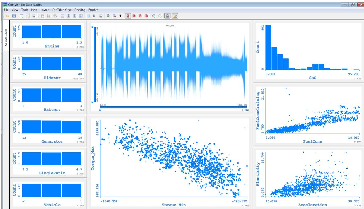
Figure 3: The coordinated multiple views system used to explore the ensemble. The six histograms on the left show the control parameters, and other views show output values.
