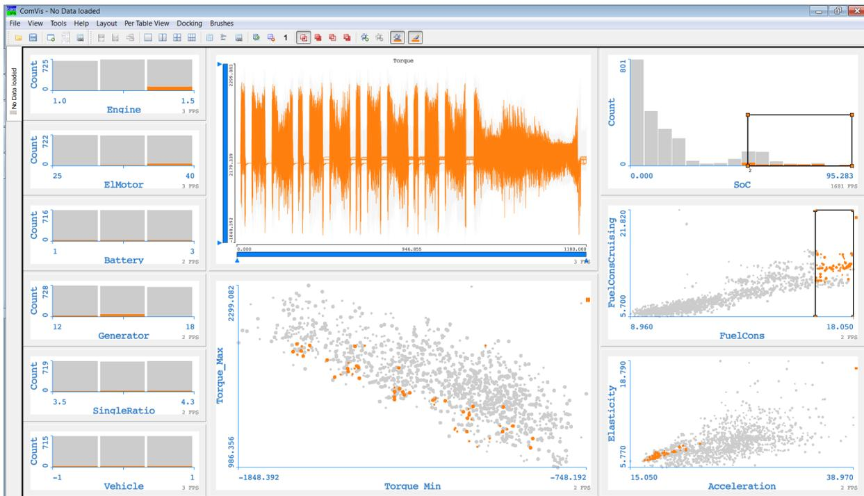
Figure 4: All views are linked—if the user selects a subset in a view all corresponding items in other views are highlighted. The user here brushes high state of charge in the upper right histogram and combines this brush with the high consumption brush from the scatter plot. All other values for selected ensemble members are highlighted in all other views.
