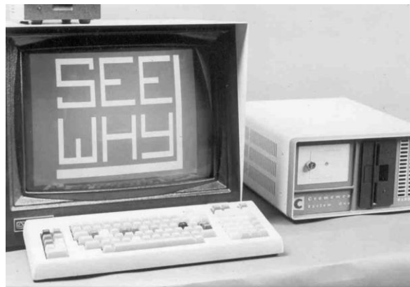
Figure 8: Typical Cromemco-based SEE WHY System.
