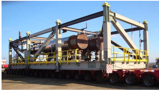
Figure 1: Typical industrial module.
