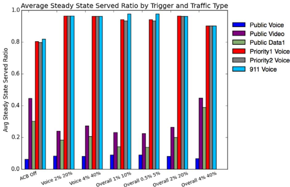
Figure 4: Steady-state ACB Trigger Comparison Summary.
