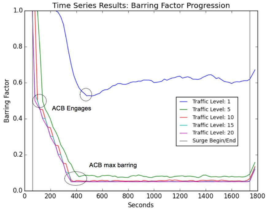
Figure 8: Barring Factor Progression over Time, for Voice 2% 20% Trigger.
