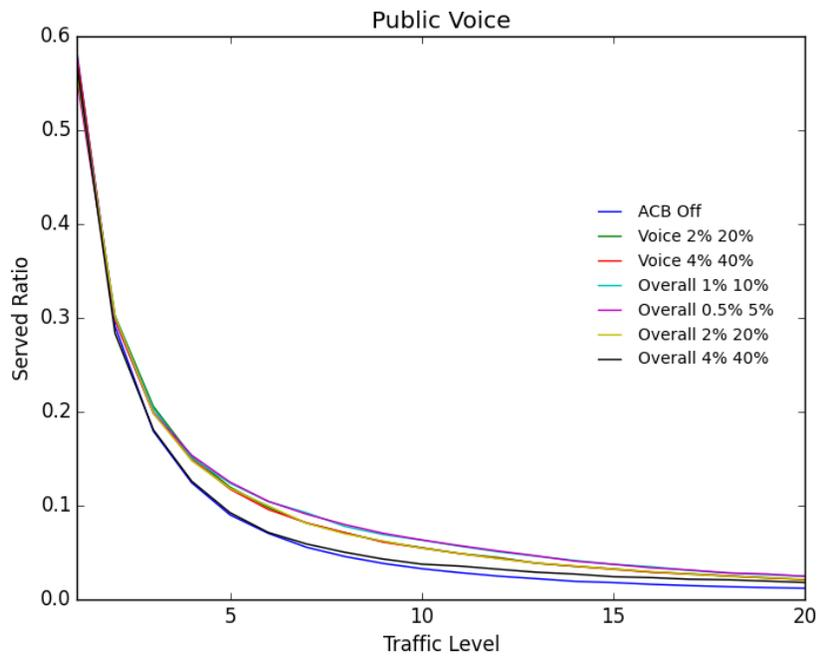
Figure 6: Steady-state ACB Trigger Comparison for Public Voice Traffic.
