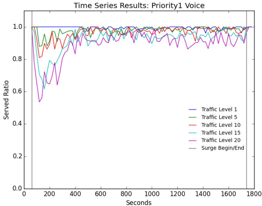
Figure 7: Transient Served Ratio for Priority1 Traffic, for Voice 2% 20% Trigger.
