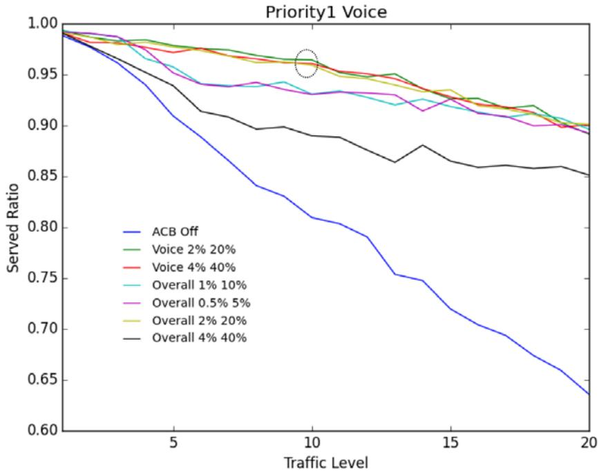
Figure 5: Steady-state ACB Trigger Comparison for Priority1 Traffic.
