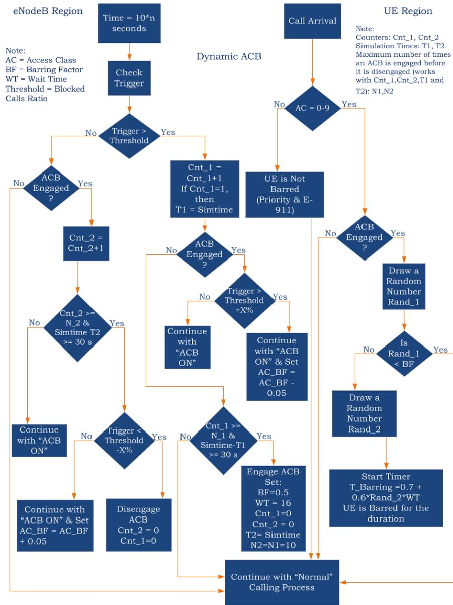
Figure 2: Access Class Barring Algorithm.
