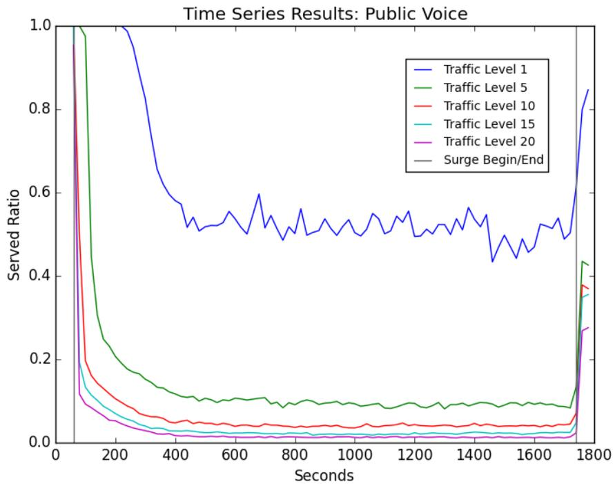
Figure 9: Transient Served Ratio for Public Voice Traffic, for Voice 2% 20% Trigger.
