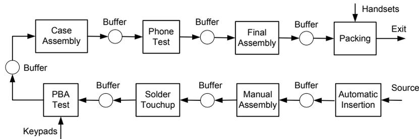
Figure 4: The manufacturing process.
