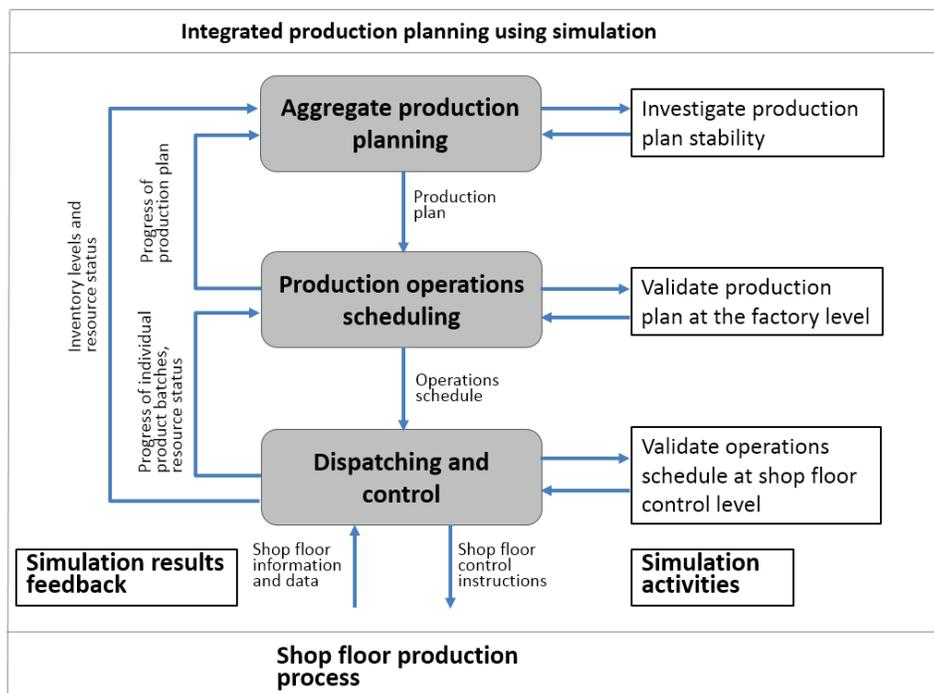
Figure 1. Simulation result feedback for integrated production planning.
