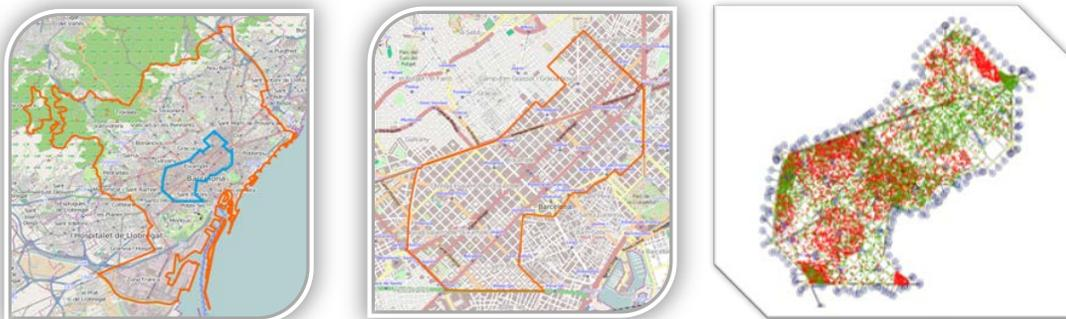
Figure 3: L’Eixample in Barcelona (left), simulation test-site (central), and the Aimsun model (right) – with spatial distribution of demand requests for the new mode in the base scenario.
