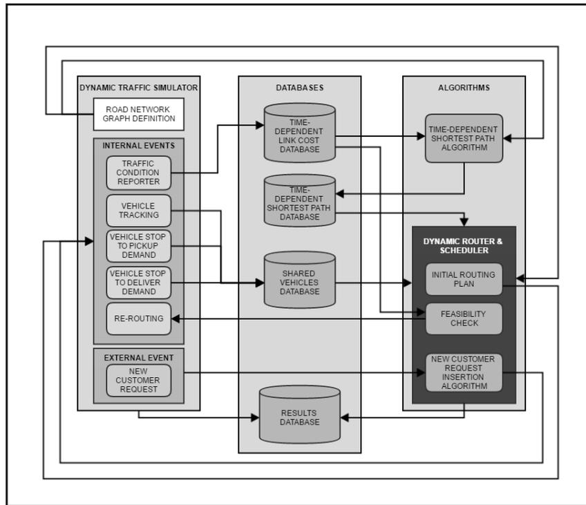
Figure 1: System Architecture.
