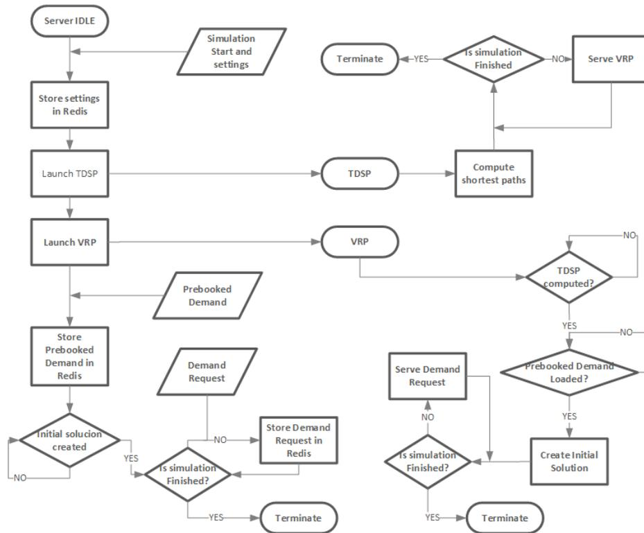
Figure 2: Flow diagram of the system process.
