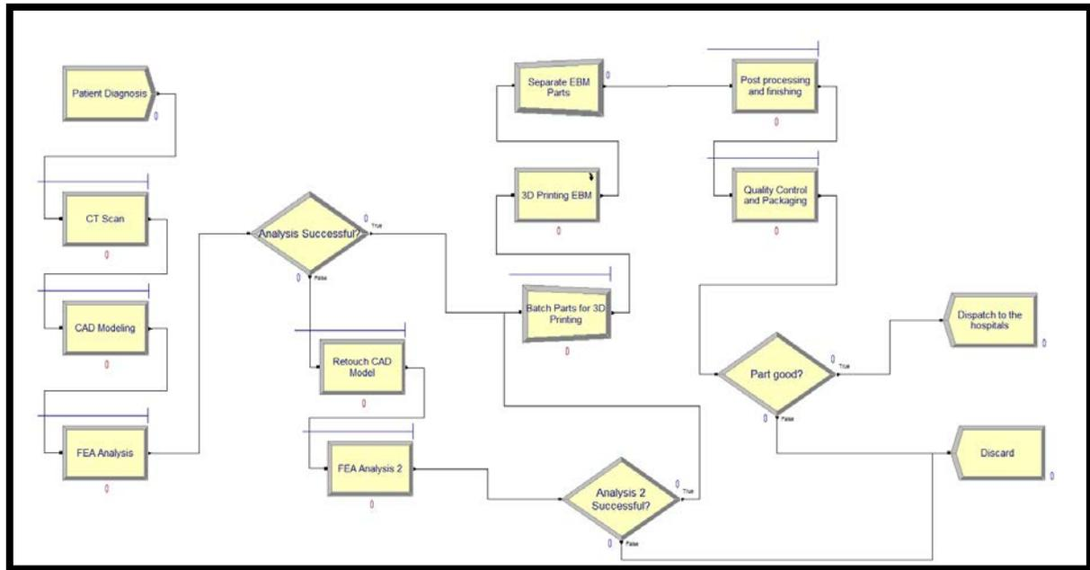
Figure 4 Simulation model for additive manufacturing of hip stems.
