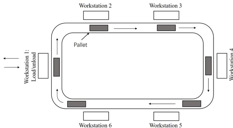
Figure 5: Closed-Loop Flexible Assembly System with six workstations and six pallets.
