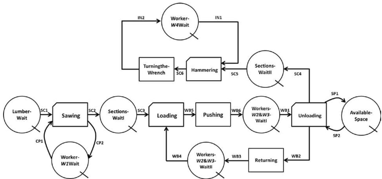
Figure 3: The ACD of the operation for modeling in Stroboscope.
