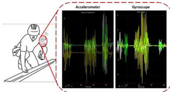
Figure 2: Different body motions create distinctive patterns in accelerometer and gyroscope data.
