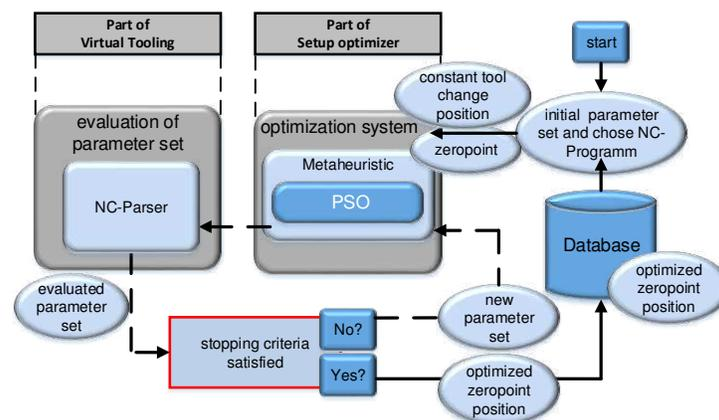
Figure 2: Schematic simulation-based optimization loop of optimizing zero point via NC-Parser interface.
