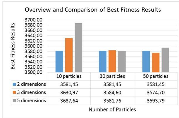
Figure 5: Overview of the comparison of best fitness results with different dimensions and particle size.
