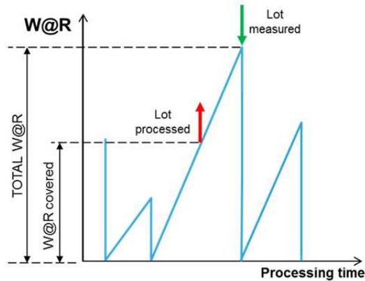
Figure 2: Wafer at risk (W@R) behavior for a process tool of Ion Implant workcenter.
