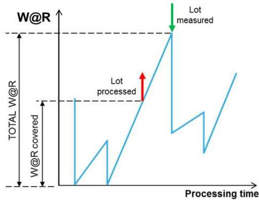
Figure 1: Wafer at risk (W@R) behavior for a process tool in the general case.
