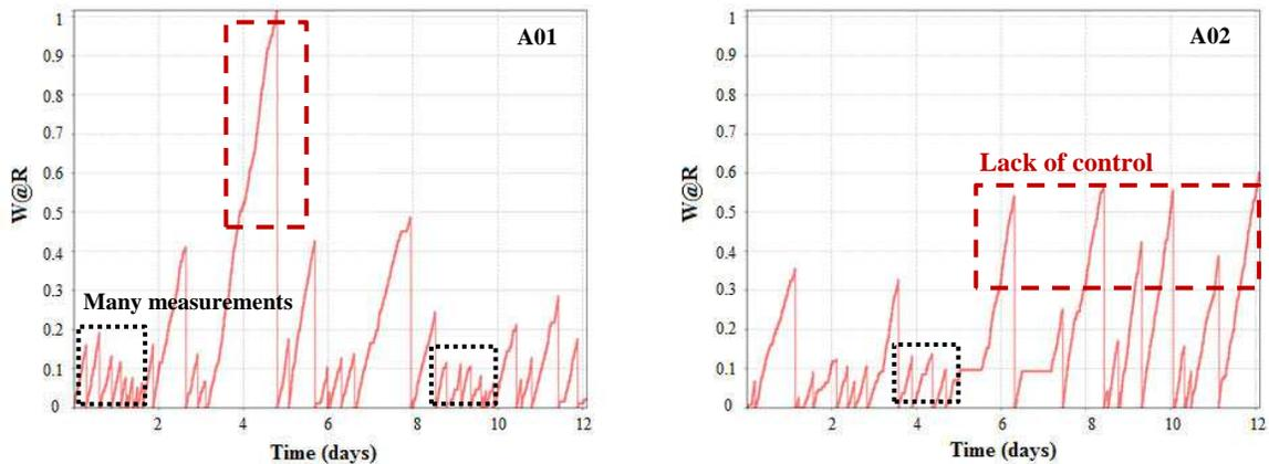
Figure 6: W@R evolution for process tools A01 and A02 for real data.
