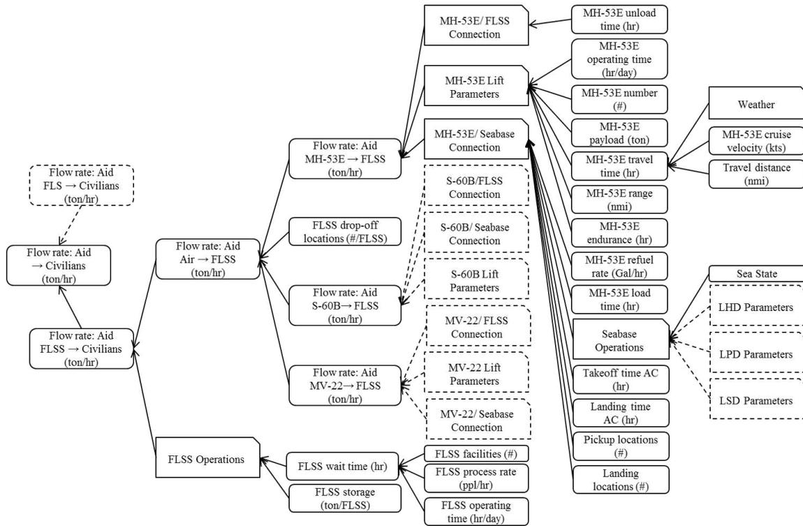
Figure 4: FLSS flow rate decomposition (MH-53E expansion L1-L7).
