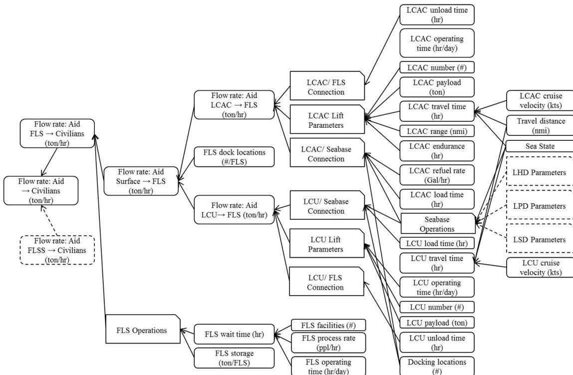
Figure 3: FLS flow rate decomposition (L1-L7).
