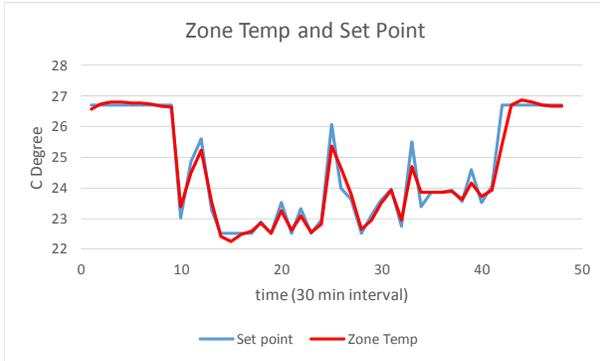
Figure 3: Optimal set point and zone temperature.
