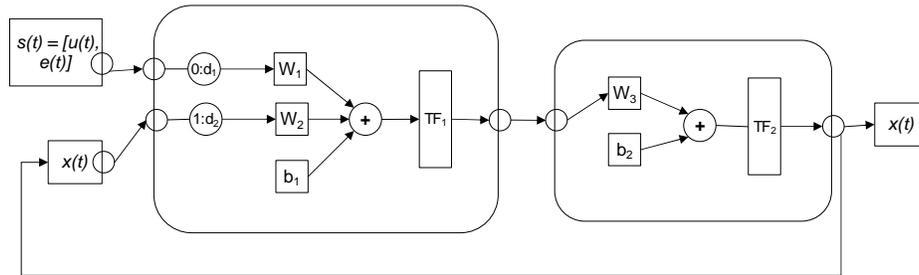
Figure 2: NARX model for thermal behavior of building.
