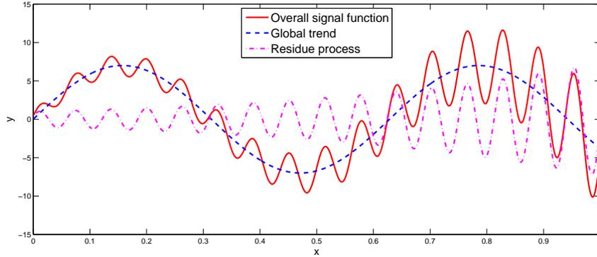
Figure 1: Decomposition of the signal function
